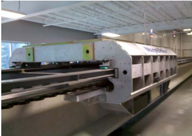
Figure 3. Test Sled mounted on indoor 48 meter Test Track at MagneMotion, Devens, MA
